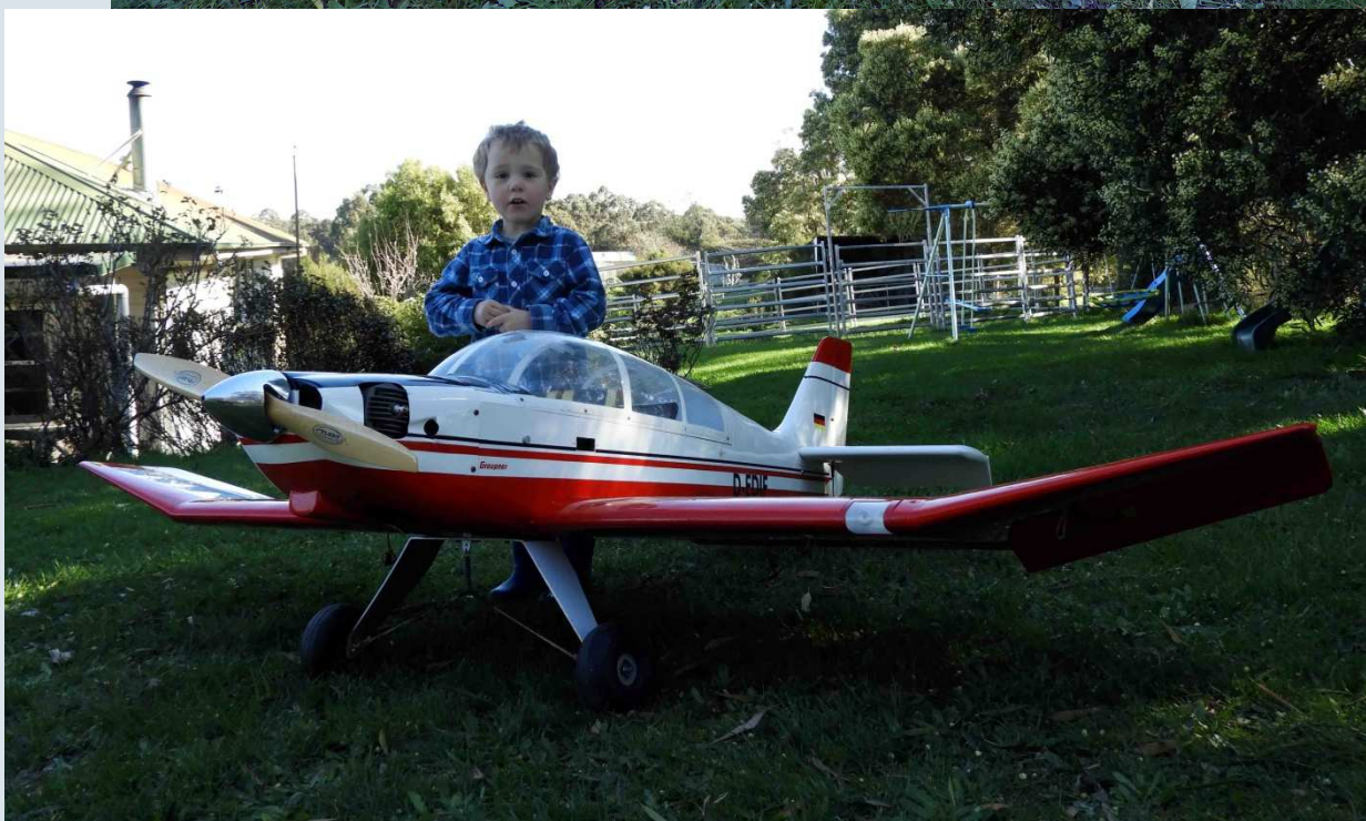
Graupner Jodel – with a Brave Heart 100 cc twin engine squeezed in for Glider Tug duties
