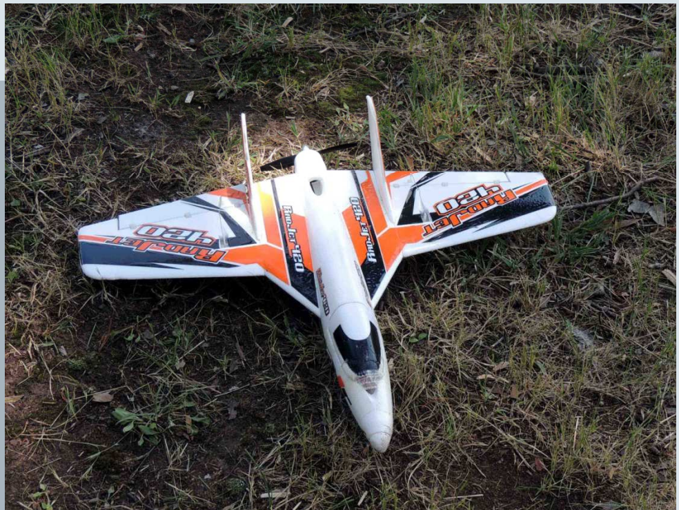
Tiny micro Delta flies on a 2 cell 300 mAh battery
